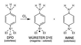
Free chlorine is measured by adding a precisely measured amount of DPD reagent to the sample, along with a pH stabilising buffer to maintain the pH between 6.3 and 6.6. Total chlorine can be measured by adding iodine and reducing the pH to 5.1.
